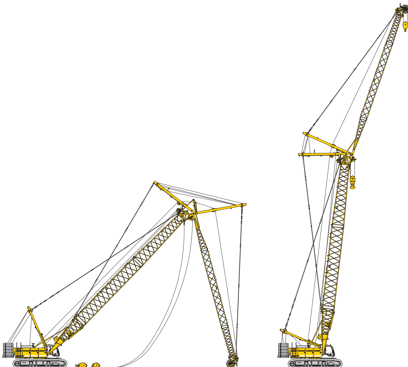
Erecting of main boom and luffing jib
