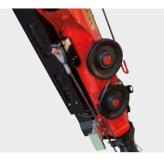
**RTC (rope tension control)** Keeps the lifting cable under tension when operating and folding winch and jib.
