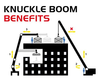
The PALFINGER knuckle boom allows the load to be positioned or lifted over a roof and inside a building with the full-powered boom, jib or optional winch. The PALcom P7 remote enables easy operation while keeping the load constantly in view for maximum safety and efficiency. In most cases no signalman is needed.
