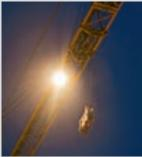
A site lighting system integrated into the jib makes it possible to work even after dark.
